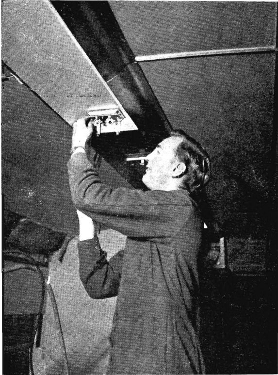
Fitting fluorescent lighting fixtures in 280 h.p. Diesel rail-car
