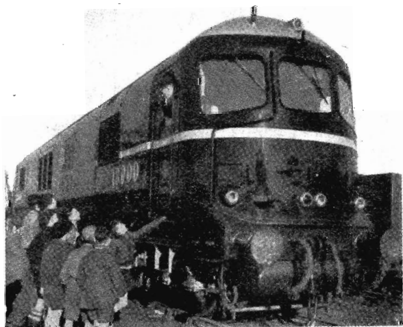
Gas turbine locomotive built by Brown-Boveri, of Switzerland, for the Western Region of British Railways, on arrival at Harwich early this year.
