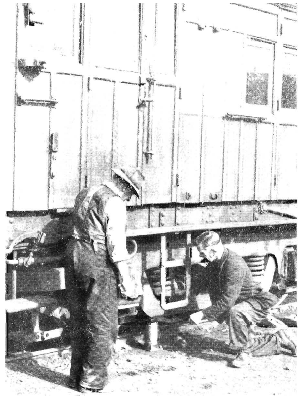
Lifting car with jack to renew wheel bearing
