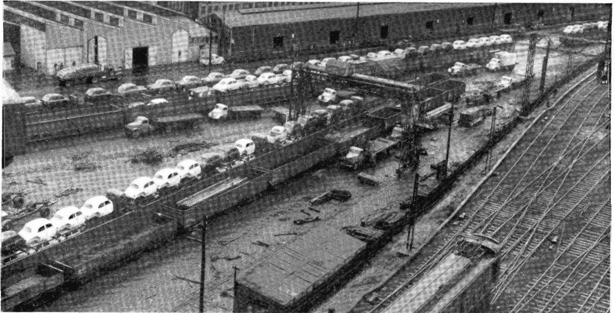
U P to forty truck loads of motor bodies are now received weekly at the Melbourne Goods Sheds from Woodville (South Australia). No. 2 gantry crane is fully occupied in unloading them, and at times the traffic is so heavy that a mobile crane has to be used also. The bodies are carried on specially built trucks. It's a six day per week service. The above picture shows a typical scene at the Sheds.
